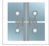
Alight façade system with external glazing fixed with grampons and fixing pieces: ball & socket or fixed. The grampons are made from stainless steel and surround the ball & socket and following this the previously machined glazing is fixed.
